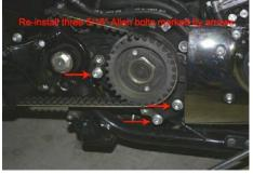
2. Replace front sprocket cover. Longer 3/16" Allen Head Bolt goes in top right hole. Lower 3/16" Allen Head Bolt will require approximately 1/8" stack of 1/4" washers to take up the space from the missing exhaust crossover tube between the cover and the engine case. Install original support bracket and RB Racing support bracket under 5/16" Allen Head Bolt.
