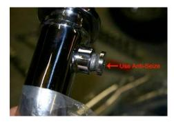
6. Install billet gaskets into the head pipes.
