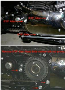
7. Remove the Exhaust crossover/support bracket using the 5/16" Allen Driver on the three allen bolts, then slip the bracket over the rear brake rod.
