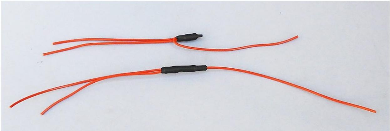
The Parallel Stub Splice has all three wires in one end and one wire loops back. This method results in the shortest splice and the best stress relief and has 3/4" of adhesive heat shrink
