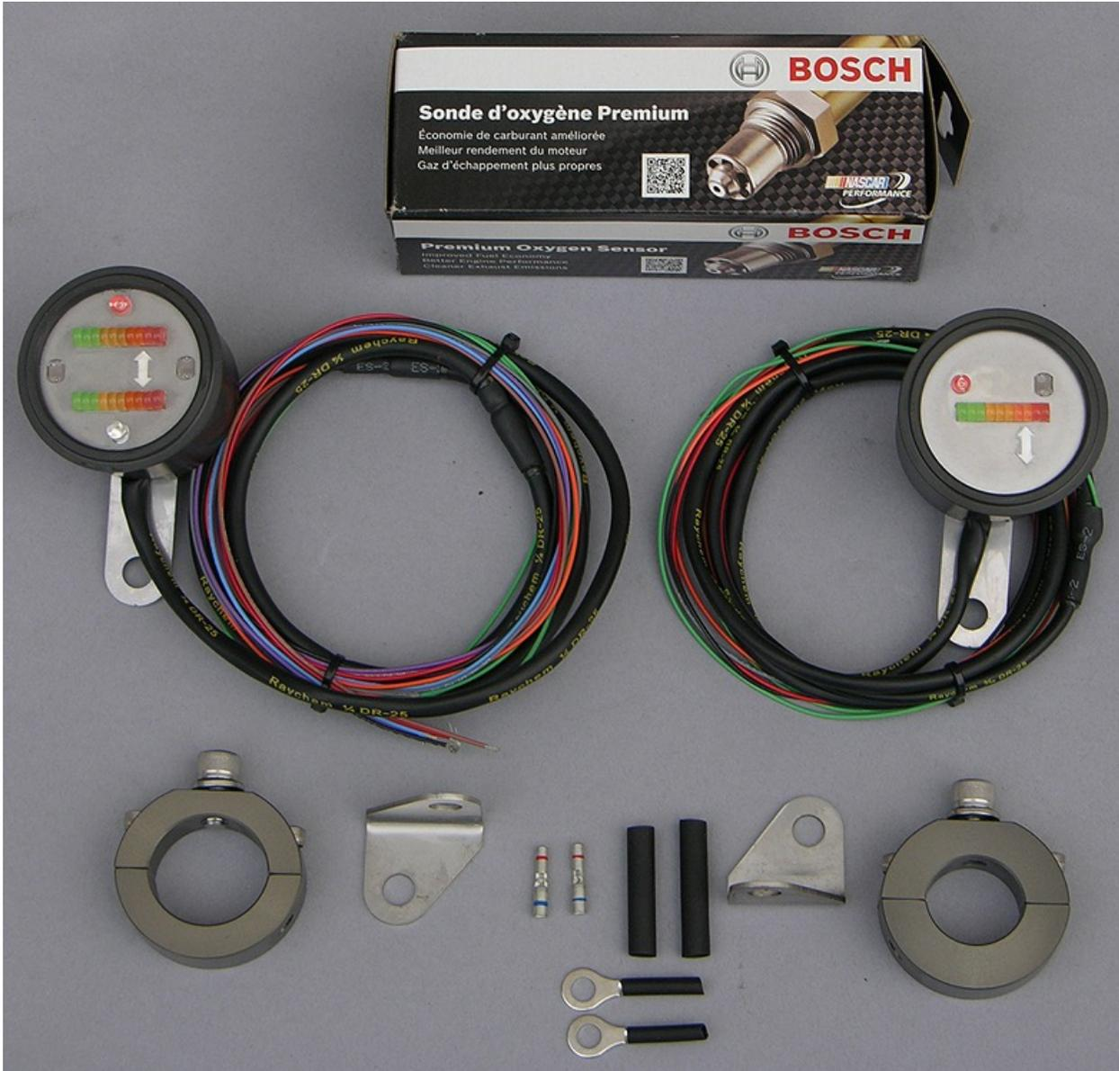
Single and Dual O2 Gauges are correctly installed when green lights are to the left as pictured.
