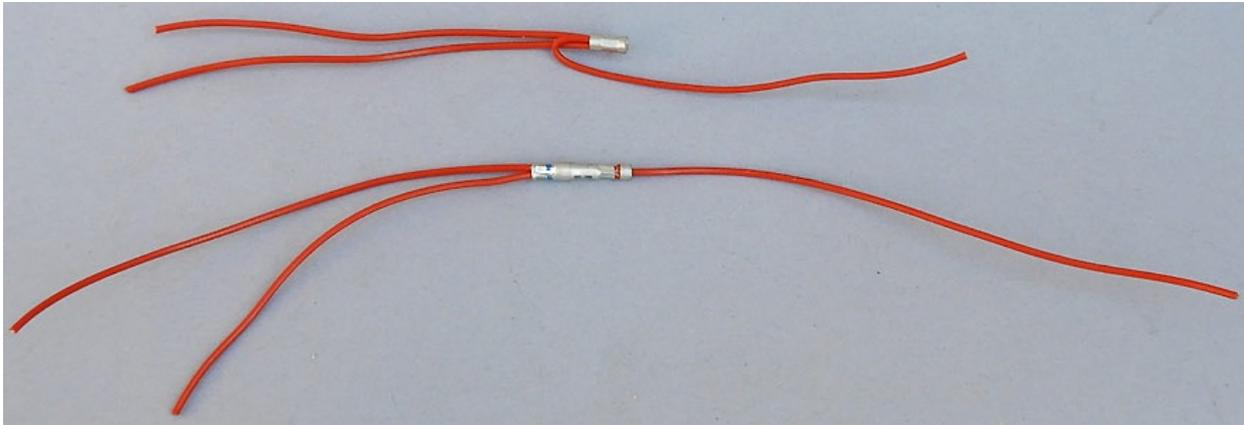
Top splice is a Parallel Stub Splice
