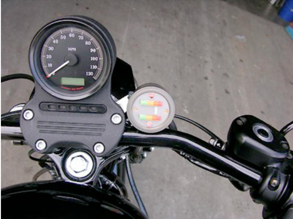
Dual O2 Meter mounted on headlight nacelle. Customer makes own bracket to back of gauge.
