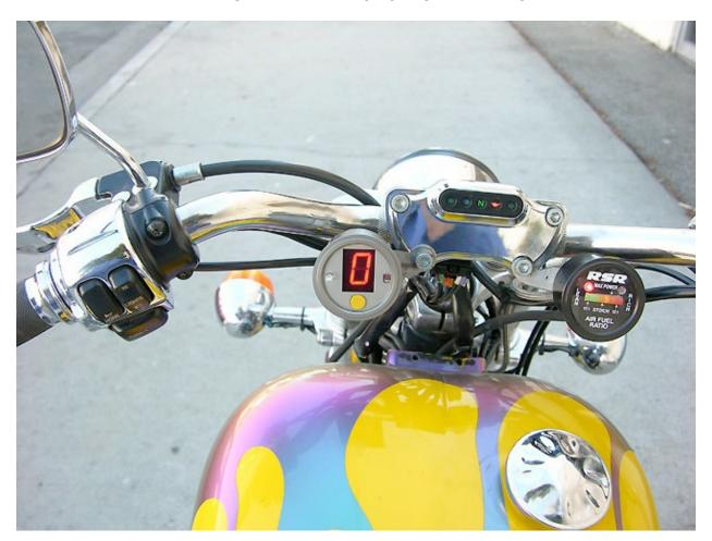
During daylight operation the display needs to be at full brightness. At night the display needs to be dimmed to avoid a blinding distraction.
