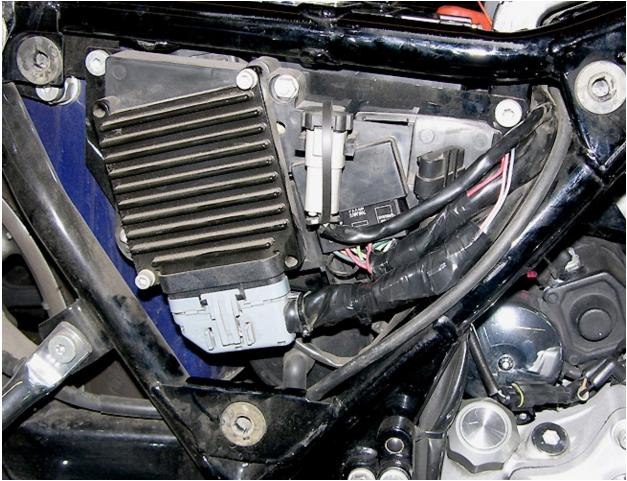
a. Blue Wire: Scotchlock to White/Green Stripe speed signal from transmission speed sensor leading to ECU. Split covering ECU harness to access the wire.Use non-adhesive harness wrap provided to cover Scotchlock on ecu harness. Wrap from "top" down and secure bottom of wrap with a plastic wire tie.
