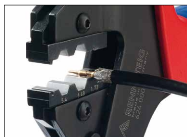
Innenleiter-Crimp Inner conductor crimp
