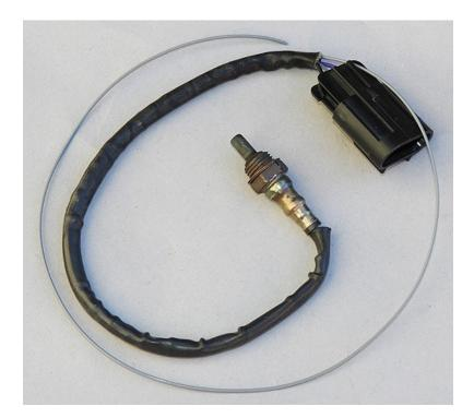
Front and rear O2 sensors must be disconnected and removed (14mm) from the bike.
