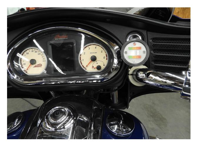
Dual O2 Gauges are correctly installed when green lights are to the left (as pictured).
