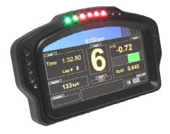
Designed to be a central part of a vehicle system, with an Ethernet hub built in, 12V or 24V systems, programmable excitations, 4 CAN ports, LIN and serial ports, 20 analogue channels, 16 digitals there is plenty of input and output capability.
