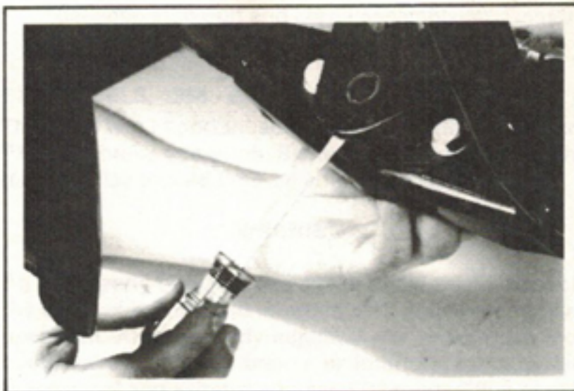
Figure 2-40. Aligning Mount Front-to-Rear
