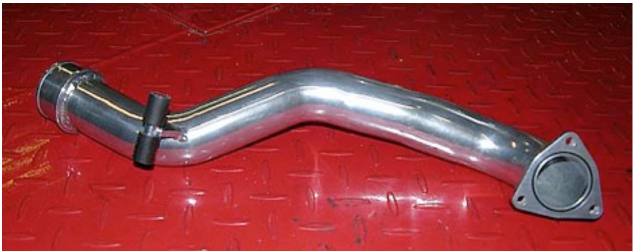
This is the turbo to intercooler ceramic coated connector pipe. Note the O-Ring in the three bolt mounting flange and the two rubber bumpers on the tube. The two rubber bumpers will press against the base of the intercooler.
