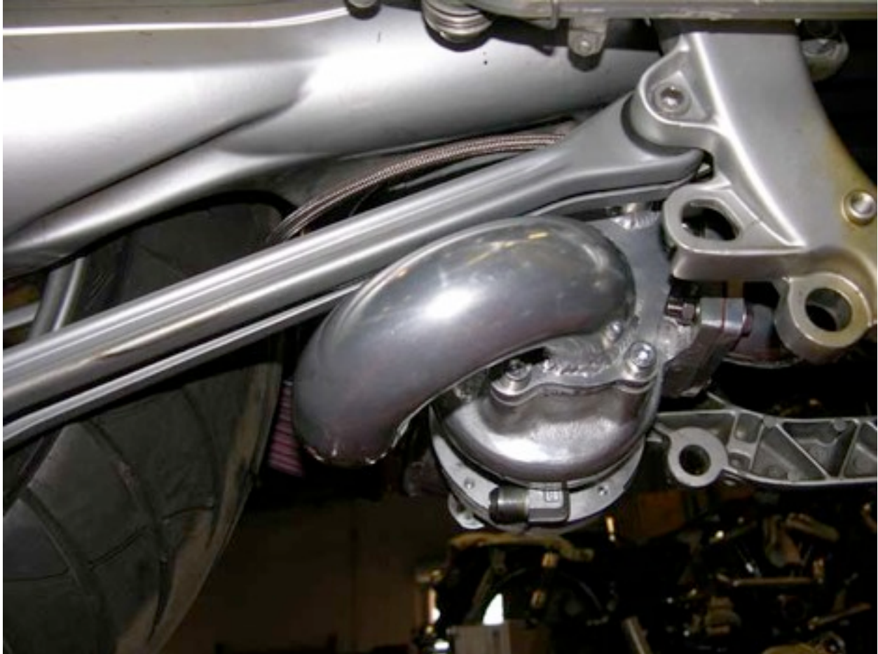
Here the stainless steel AN4 oil feed line passes over the 10mm mounting bolt location
