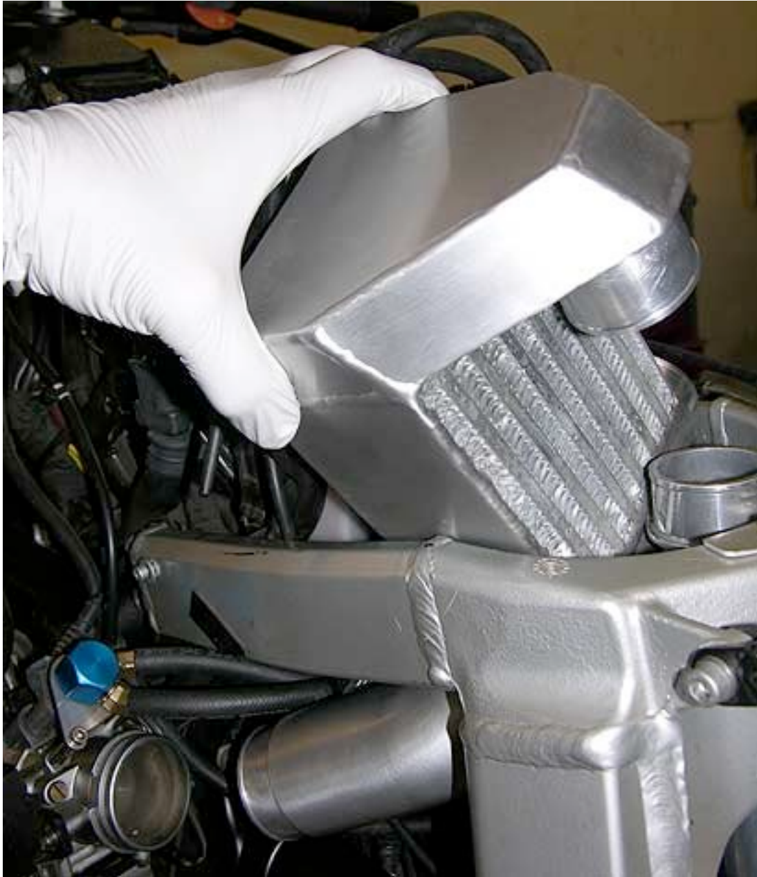
The intercooler is inserted from the top.
