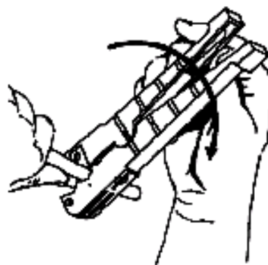
Figure 13. Coaxial Cable Stripping
