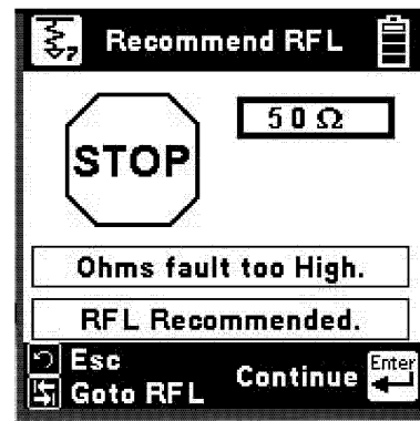
Figure 26. AST900 Resistance Fault Display Auto TDR operates from a captured trace. The trace is not 'live' as in the standard TDR mode.
