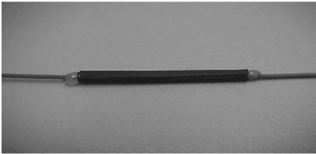
Figure 27. Completed Wrap-Around Heat Shrink Repair on Single Conductor
