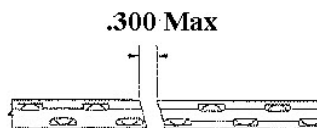
45° cuts at "terminal" ends for staggered type (NASM22529/2) caterpillar grommets
