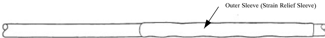
Figure 34. Double Shield Twin Axial Cable Repair with Solder Sleeve Primary Splice (Sheet 2 of 2)
