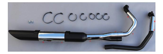
Remove the OEM exhaust system...4mm Allen to remove finned exhaust port covers; 8mm Allen to loosen and lower right floorboard (support underneath to reduce strain on brake line); Unplug (2) O2 sensors. Remove left and right side exhausts...Various Metric sockets.
