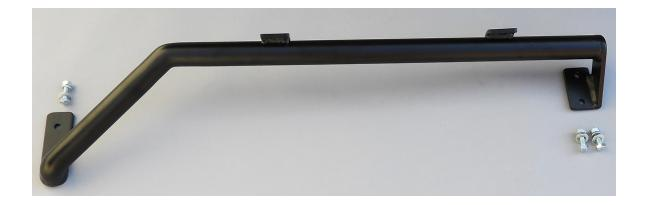
The left side support bar is secured by (3)  $8mm \times 1.25 \times 25mm$  bolts; (3) 8mm flat washers; (3) 8mm split lock washers; (3)  $8mm \times 1.25$  hex nuts. Washer under bolt head. Bolts from outside facing "in" towards the motorcycle. Lock washer and nut to the inside.
