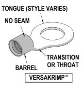
allows for crimping from any direction without the barrel opening up, and provides greater tensile strength. This terminal is ideal for hard to crimp solid and stranded wires. It is available in wire range 4/0 to 22 AWG (0.10 to 117.00mm<sup>2</sup>).
