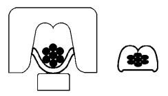
The <u>Confined crimp</u> gives the best overall crimp. It is in the shape of a hexagon, an enclosed "C", or a confined quad. The advantages of all three crimps are uniformity and compression of individual strands and uniform outer appearance.
