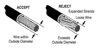
Check the insulation to ensure that there has been a nice clean cut. Wires with damaged insulation should not be used.
