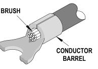
contact side of the terminal. This helps ensure that mechanical compression occurs over the full length of the conductor crimp. The conductor brush should not extend into the contact area.
