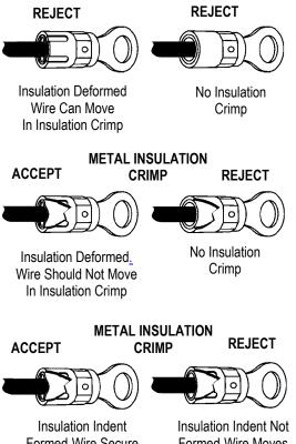
Formed-Wire Secure In Insulation Crimp
