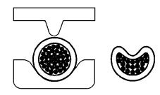
The <u>F crimp</u> is used to close the barrel and confine the individual strands. The overall quality is excellent.
