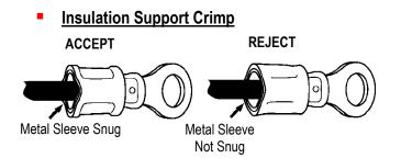
On closed barrel terminals that have a secondary metal sleeve (AviKrimp<sup>™</sup>), the metal sleeve should be formed snugly around the wire.
