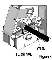
6. Inspect for proper crimp location. Check the Air Powered Crimp Hand Tool Specification Sheet that you are using for correct conductor crimp height
