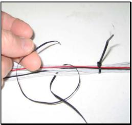
Start by loosely placing a tie wrap around the harness. As you tie lacing cord around the harness, you will slide the tie wrap along the harness to help keep the wires neatly combed together.
