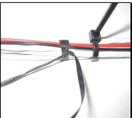
After the ends are tied, cut the ends off leaving about ¼ inch of cord.
